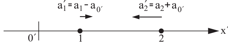
Figure 14.2: Accelerations a'_1 and a'_2 of two bodies relative to a frame of reference O' .
